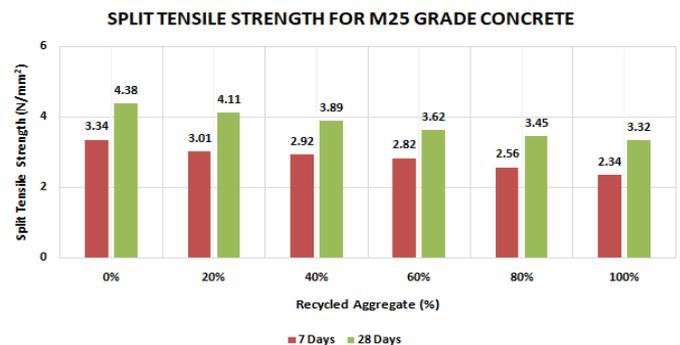
**Chart 6:** Split Tensile Strength for varying % of RCA for M<sub>30</sub> Grade Concrete
